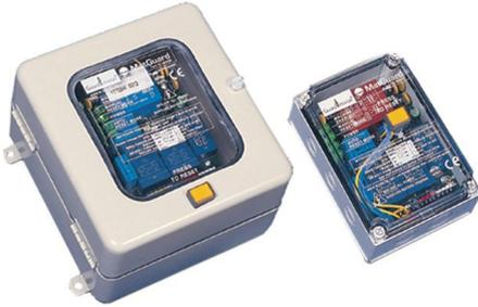
The controller detects a presence on the mat, a short circuit, or an open circuit. Under each of these conditions, the safety output relays turn off. When interfaced properly, the machine or hazardous motion will receive a stop signal, and an auxiliary output relay turns ON.
