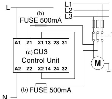
(d) The CU3 monitors the connections to the motor via the Z1-Z2 terminals. A break in the Z1-Z2 loop will be detected and the safety output contacts 13-14 & 23-24 will be prevented from closing when the motor is either running or stopped. To restore the CU3 function: isolate all power, repair the fault in the Z1-Z2 loop and reinstate power. Check for correct operation.
