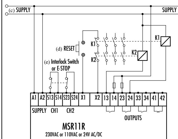
(f) The supply voltage must meet the requirements of EN 60204-1. Terminal A2 must be connected to that side of the control circuit which is connected to the protective conductor.
