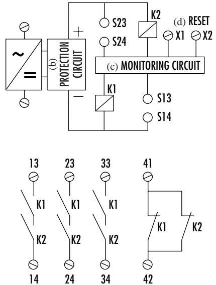
**5 (a) Wiring example / Anschlußbeispiele / Exemples de câblage****(b) Interlock Switch or E-STOP control with Monitoring of External Relays with Monitored Reset.**
