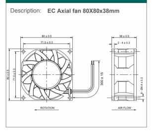
Casing material: Impeller material Protection degree: Fixing system: Motor protection: Lifetime L10 at 25°C: Electrical connection: Approvals: Weight: Thermoplastic in black color, UL 94 V-0 Thermoplastic in black color, UL 94 V-0 IP20, according to EN 60529 standard by No 4 M4 screws Impedance 50,000 h 2 leads 24 AWG UL1430 CE 0.270 kg
