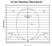
Note: There must be a minimum spacing of 4 mm (0.157 in) if actuator and sensor face approaches laterally. This will prevent false triggering due to the side lobe areas.
