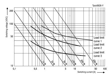
Load limit curve 1  $\triangleq$  safe shutdown, connected as form X, load on pin 5 and 7
