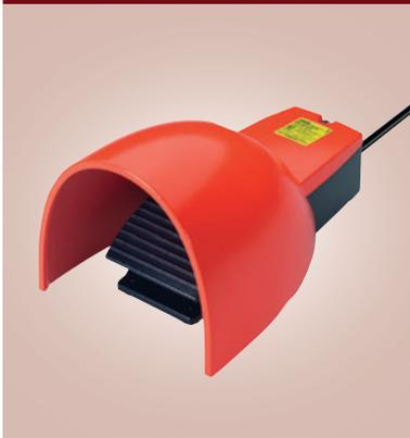
An explosion proof foot switch with protective shield certified for use in Ex zone 1 and 2 as well as dust groups 21 and 22. Snap action contacts also available. For category Ex dust zone 22 ask for suffix 3D version.
