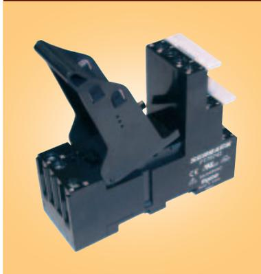
DIN rail mounting sockets suitable for Schrack 4 pole 14 pin PT series relays. Sockets are designed so that coil connections are at one end, and all other connections are at the other end of the socket to aid wiring separation. Sockets are IP20 finger proof and accept diode, led and protection modules from standard socket.
