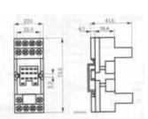
DIN rail mounting sockets suitable for Schrack PT series relays. Sockets are IP20 finger proof and rated to match the relay.
