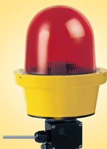
An Explosion proof double flash xenon beacon suitable for use in Ex zones 1 and 2 as well as dust zones 21 and 22. This model has a 15 Joule flash energy and has a life expectancy of 4 million flashes at 1 Hz. Alternative tube mounting brackets available as is a protective wire guard.
