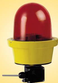
An Explosion proof LED rotating beacon suitable in EX zones 1 and 2 as well as dust zones 21 and 22. The rotating effect is created by electronics without the need for moving parts. This model has a 50000 hour life expectancy. Alternative tube mounting brackets available as is a protective wire guard.
