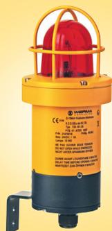
A compact explosion proof flashing beacon suitable for use in Ex zones 1 and 2. This model has a 15 Joule flash energy and has a life expectancy of 4 million flashes at 1 Hz. Integral protective wire guard and bracket.
