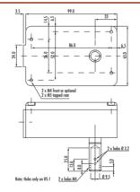
The Rotacam is a robust heavy duty rotary actuated safety switch designed to fit at the hinge point of guards. The shaft is strong enough to be utilised as, or connected to, the existing hinge pin. Switch isolates power with just 5° of door movement, adjustable cam allows switching adjustment to 11°. Available with 2 N/C safety contacts + 1N/O auxiliary contact
