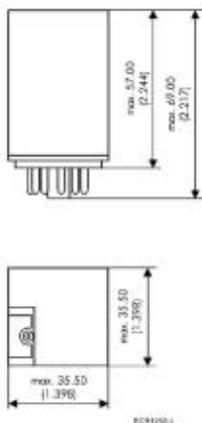
A universal 11 pin 3 pole change over relay rated to 10A. The relays feature a mechanical flag and test lever as standard. LED indication, gold plated or bifurcated contacts and other voltages available on request.
