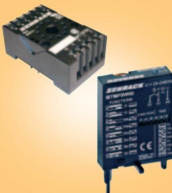
DIN rail mounting IP20 sockets for 11 pin relays. The multifunction version is designed to accept a timer module. The multifunction timer provides a wide variety of timing functions from 0.05 S to 240 hours such as delay on, delay off, single hot, flashing and so on. Its supply voltage range is 24 to 240V ac or dc.
