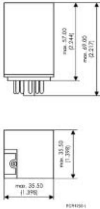
A universal 8 pin 2 pole change over relay rated to 10A. The relays feature a mechanical flag and test lever as standard. LED indication, gold plated or bifurcated contacts and other voltages available on request.
