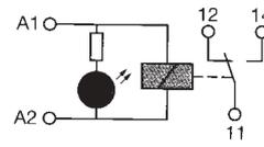
Slimline relay for DIN rail mounting with SPCO contacts rated to 6A at 400V ac. 6mm width. Relay status indication by LED. Integrated diodes for coil suppression and polarity protection.
