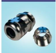
The *PERFECT* range of high quality EMC safe cable glands, suitable for screened cables. Easy to assemble, the shield of the cable is pressed down with the plastic insert to the floor of the gland. When used with locknuts with cutting edges (supplied separately), it will provide potential compensation with optimal contact.
