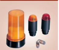
A amber static light beacon lamp with a 20mm conduit thread which will screw into conduit entries. Ideal for indication of switch state when wired to an auxiliary contact of a switch. Available with 24, 110 or 230 volt lamps.
