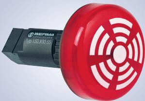
A permanent led combined with an electronic buzzer suitable for 22.5mm panel mounting. 2800Hz continuous tone. High output of 80db at 1m.
