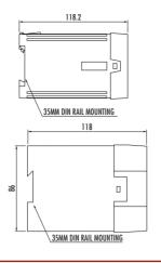
The MSR10RD 'Minotaur' is a dual channel input safety relay with multiple supply voltages and immediate and delayed outputs especially useful for use with PLC control machines. It monitors contactors, input devices and PLC safety functions. With fail-safe internal monitoring and monitored manual reset, any single detected fault will result in lock-out to a safe state. Featuring 8 N/O + 1N/C outputs and 1 N/O + 1 N/C time delay outputs, internally adjustable from 0.1-10 seconds.
