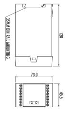
The MSR15RD 'Minotaur' is a dual channel input safety relay with immediate and delayed outputs especially useful for use with PLC control where power must be partially maintained for an active braking sequence, after which all power must be removed. Features 2 N/O + 1N/C instantaneous outputs and 1 N/O off delay output, internally adjustable from 0.1-10 seconds.
