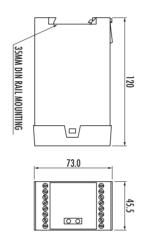
The MSR11R 'Minotaur' is a dual channel input safety relay featuring a monitored manual reset function which prevents loop-out defeating of the reset button. Any attempt at defeat will resulting in lock-out of relay. Available in three voltage versions.
