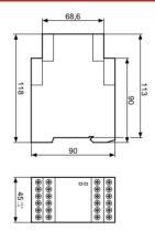
The KZH3-RS is a two hand control device that can receive the following components as inputs: two pushbuttons with two positions "N/O + N/C", one or two emergency stop pushbuttons with one or two channels. The number of contacts of the KZH3-RS can be extended and the breaking capacity increased when used with the KZE3-XS.
