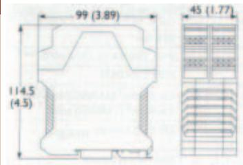
The MSR138.1 safety relay has a set of 2 N/C immediate safety outputs and a second set of 2 N/O and 1 N/C safety outputs which may be delayed. The relay can be connected to 3 possible input configurations: 1 N/C safety contact, 2 N/C safety contact or 2 pnp light curtain outputs. Automatic or monitored manual reset. These units feature removable terminal blocks.
