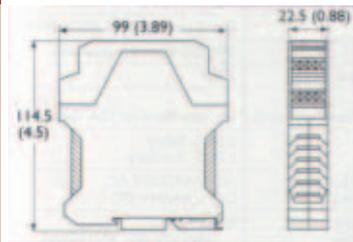
The MSR125HP relay may be used to interface to two hand control devices. The relay requires that the 2 input switches operate within 0.5 seconds of each other and will only authorise an on condition whilst both are held down. If one of the switches is released the machine cannot be restarted until both switches have been released.
