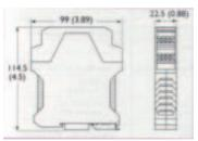
The MSR125HP relay may be used to interface to two hand control devices. The relay requires that the 2 input switches operate within 0.5 seconds of each other and will only authorise an on condition whilst both are held down. If one of the switches is released the machine cannot be restarted until both switches have been released.
