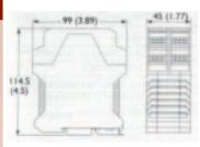
The MSR138.1 safety relay has a set of 2 N/C immediate safety outputs and a second set of 2 N/O and 1 N/C safety outputs which may be delayed. The relay can be connected to 3 possible input configurations: 1 N/C safety contact, 2 N/C safety contact or 2 pnp light curtain outputs. Automatic or monitored manual reset. These units feature removable terminal blocks.
