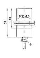
An explosion proof magnetically operated reed switch housed in an M30 threaded stainless steel body. Switch will only operate by proximity to a matching coded magnet. Overide by an ordinary magnet is therefore prevented making this device suitable for safety applictions. The reed switches are internally limited by a 20 ohm resistor to ensure contacts cannot be overloaded. Magnets supplied separately. M16 mounting thread also available.
