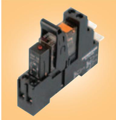
A din rail socket suitable to mount relays with 5mm pinning from the XT range of relays. Can be used with double pole or single pole relay. Note socket is rated to 12A per terminal. If using full 16A of single pole relay rating ensure terminals 11-21, 12-22 and 14-24 are bridged to enhance the rating. Available with a retaining clip to hold relay in place and a variety of protection and indication modules.
