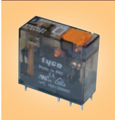
The XT series relays are a new generation of plug in relays featuring a clear case and extra strong pins for greater mechanical strength. Also features a manual test lever as standard and a sensitive 400mW coil with built in led indication and suppression diode. Suitable for RT series DIN rail sockets.
