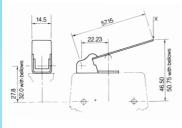
A general purpose double pole snap action miniswitch with double make double break contacts (commoning link enables 1 changeover). Supplied with a 14.5 x 57.15mm phosphor bronze plain lever. Screw terminals, entry via 13.5mm conduit hole.
