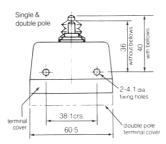
A general purpose single pole snap action miniswitch with double make double break contacts (commoning link enables 1 changeover). Supplied with plunger and neoprene bellows. Screw terminals.
