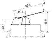
A medium duty single pole snap action miniswitch with double make double break contacts (commoning link enables 1 changeover). Supplied with a 14.5 x 57.15mm phosphor bronze plain lever and plunger with neoprene bellows. Screw terminals, entry via M16 tapped conduit hole.
