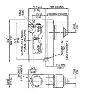
A single pole snap action changeover microswitch enclosed in an aluminium housing certified for use in zone 1 or zone 2. For zone 1, installation must be in accordance with code of practice BS5346, part 6 and cable glands to BS6121 (except types A1, A3 and B) must be fitted. Cowled standard plunger actuator offering IP67 protection.
