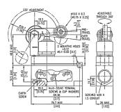
A single pole snap action changeover microswitch enclosed in an aluminium housing certified for use in zone 1 or zone 2. For zone 1, installation must be in accordance with code of practice BS5346, part 6 and cable glands to BS6121 (except types A1, A3 and B) must be fitted. Available with a cowl protected roller lever adjustable through 360° horizontally and 235° vertically. M20 conduit entry to screw terminals.
