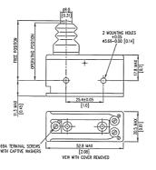
Two plastic case single pole changeover, snap action switches featuring enclosed screw terminals with access via a removable insulated cover. Cowled plunger and sealed to either IP54 or IP67 (except terminals).
