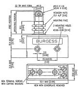
A hole mounted metal case single pole changeover, snap action switches featuring enclosed screw terminals with access via a removable insulated cover. Available with a roller plunger actuator.
