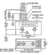
A hole mounted metal case single pole changeover, snap action switches featuring enclosed screw terminals with access via a removable insulated cover. Available with a plain plunger actuator.
