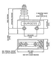
Two metal case single pole changeover, snap action switches featuring enclosed screw terminals with access via a removable insulated cover. Cowled plunger and sealed to either IP54 or IP67 (except terminals). Also available with a flat long auxiliary actuator, please order separately.
