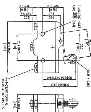
A single pole, snap action, changeover microswitch incorporating a beryllium copper trident spring mechanism, silver contacts and accessible screw terminals. Featuring a 26.7 mm roller lever actuator.
