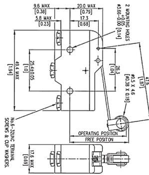
A single pole, snap action, changeover microswitch incorporating a beryllium copper trident spring mechanism, silver contacts and accessible screw terminals. Featuring a 48.2 mm roller lever actuator.
