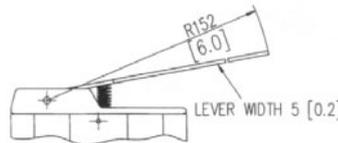
A single pole, snap action, changeover microswitch incorporating a beryllium copper trident spring mechanism, silver contacts and accessible screw terminals. Featuring a 152 mm plain lever actuator.
