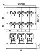
Two five way key exchange unit which allows the controlled release of keys in a interlock sequence. Primary key in/four secondary keys out. Manufactured with stainless steel interlocking and coded parts, including coded barrel & internal components. Other key code options can be supplied upon request.
