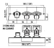
A three way key exchange unit which allows the controlled release of keys in a interlock sequence. Primary key in/two secondary keys out. Manufactured with stainless steel interlocking and coded parts, including coded barrel & internal components. Other key code options can be supplied upon request.
