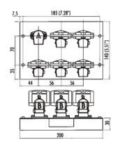
A four way key exchange unit which allows the controlled release of keys in a interlock sequence. Primary key in/three secondary keys out. Manufactured with stainless steel interlocking and coded parts, including coded barrel & internal components. Other key code options can be supplied upon request.
