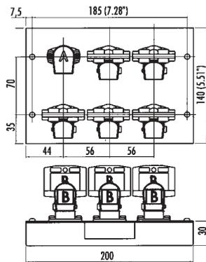
Two five way key exchange unit which allows the controlled release of keys in a interlock sequence. Primary key in/four secondary keys out. Manufactured with stainless steel interlocking and coded parts, including coded barrel & internal components. Other key code options can be supplied upon request.
