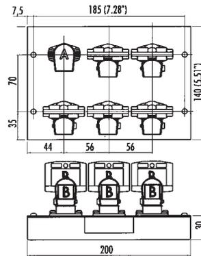
A four way key exchange unit which allows the controlled release of keys in a interlock sequence. Primary key in/three secondary keys out. Manufactured with stainless steel interlocking and coded parts, including coded barrel & internal components. Other key code options can be supplied upon request.
