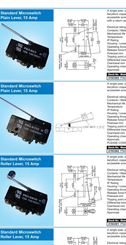
A single pole, snap action, changeover microswitch incorporating a beryllium copper trident spring mechanism, silver contacts and accessible screw terminals. Featuring a 63.5 mm plain lever actuator with a return spring.
