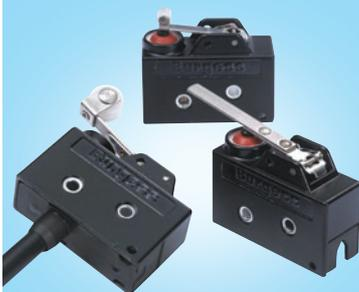
Single pole, snap action miniature microswitches which are sealed to IP67. Sturdy construction for long life in difficult environments, featuring a die cast housing. Pre-wired or screw terminals versions with plunger, plain or roller levers.
