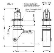
A protected miniature microswitch with a single pole changeover contact in a M10 threaded barrel sealed to IP57. Featuring a plain plunger actuator and supplied pre-wired with 0.5M PVC cable.
