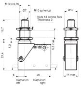
A protected miniature microswitch with a single pole changeover contact in a M10 threaded barrel sealed to IP57. Featuring a plain plunger actuator and supplied pre-wired with 0.5M PVC cable
