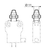
A metal enclosed safety limit switch sealed to IP67 and pre-wired with 1 metre of armoured cable. With 1 N/O + 1 N/C positive break action changeover contacts. Featuring a metal plunger actuator with threaded barrel. Longer cable lengths can be supplied, please consult sales.
