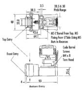
Slamlock single key is an access interlock which traps the actuator until insertion and rotation of the key. Featuring all stainless steel interlocking and coded parts, including coded barrel & internal components. Suitable for partial body access. Available in six different key code options A to F. Other key code options can be supplied upon request.
