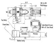
Slamlock dual key is an access interlock which traps the actuator until insertion and rotation of the key. Featuring all stainless steel interlocking and coded parts, including coded barrel & internal components. Suitable for full body access with one key in/one key out, enabling operator to use secondary key as a personnel key, to avoid being locked in. Other key code options can be supplied upon request.
