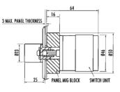
A panel mounted 4 pole, 20 Amp rotary key switch to be used for the electrical isolation of machinery to enable safe access. Key trapped/switch on, key free/switch off with 2 N/O + 2 N/C contacts. Featuring all stainless steel interlocking and coded parts, including coded barrel & internal components. High visibility traffalite label. Available in six different key code options A to F. Other key code options can be supplied upon request.
