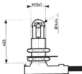
A precision movement detector with a single pole changeover contact in a M16 threaded barrel sealed to IP56. Featuring a roller plunger actuator and supplied pre-wired with 1M PVC cable.
