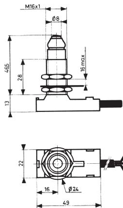
A precision movement detector with a single pole changeover contact in a M16 threaded barrel sealed to IP66. Featuring a plain plunger actuator and supplied pre-wired with a single pole changeover contact.
