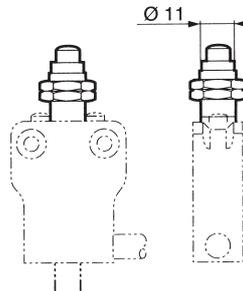
A metal enclosed safety limit switch sealed to IP67 and pre-wired with 1 metre of armoured cable. With 1 N/O + 1 N/C positive break action changeover contacts. Featuring a metal plunger actuator with threaded barrel. Longer cable lengths can be supplied, please consult sales.
