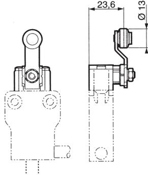
A metal enclosed safety limit switch sealed to IP67 and pre-wired with 1 metre of armoured cable. With 1 N/O + 1 N/C positive break action changeover contacts. Featuring a offset lever actuator with left and right action and steel roller actuator. Longer cable lengths can be supplied.
