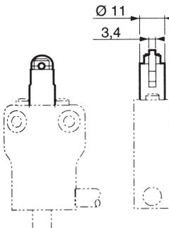
A metal enclosed safety limit switch sealed to IP67 and pre-wired with 1 metre of armoured cable. With 1 N/O + 1 N/C positive break action changeover contacts. Featuring a steel roller plunger actuator.
