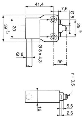
A metal enclosed safety limit switch sealed to IP67 and pre-wired with 1 metre of armoured cable. With 1 N/O + 1 N/C positive break action changeover contacts. Featuring a plain metal plunger actuator.
