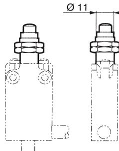
A metal enclosed safety limit switch sealed to IP67 and pre-wired with 1 metre of armoured cable. With 1 N/O + 1 N/C positive snap acting changeover contacts. Featuring a metal plunger actuator with threaded barrel.
