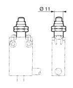
A metal enclosed safety limit switch sealed to IP67 and pre-wired with 1 metre of armoured cable. With 1 N/O + 1 N/C positive snap acting changeover contacts. Featuring a metal plunger actuator with threaded barrel.
