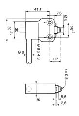
A metal enclosed safety limit switch sealed to IP67 and pre-wired with 1 metre of armoured cable. With 1 N/O + 1 N/C positive break action changeover contacts. Featuring a plain metal plunger actuator.
