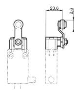
A metal enclosed safety limit switch sealed to IP67 and pre-wired with 1 metre of armoured cable. With 1 N/O + 1 N/C positive break action changeover contacts. Featuring a offset lever actuator with left and right action and steel roller actuator.
