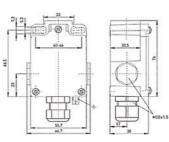
An explosion proof metal bodied limit switch. Although wider than the DIN50041 sizes the fixing hole centres are the same at 30mm separation. Dual certified for Ex zones 1 and 2 as well as dust zones 21 and 22. Slow action positive break contacts. Available also with 2 N/C positive break contacts and 1 N/O / 1 N/C overlapping positive break.
