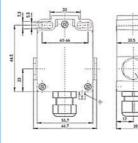
An explosion proof metal bodied limit switch. Although wider than the DIN50041 sizes the fixing hole centres are the same at 30mm separation. Dual certified for Ex zones 1 and 2 as well as dust zones 21 and 22. Slow action positive break contacts. Available also with 2 N/C positive break contacts and 1 N/O / 1 N/C overlapping positive break.
