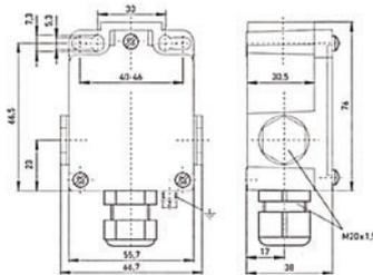
An explosion proof metal bodied limit switch. Although wider than the DIN50041 sizes the fixing hole centres are the same at 30mm separation. Dual certified for Ex zones 1 and 2 as well as dust zones 21 and 22. Slow action positive break contacts. Available also with 2 N/C positive break contacts and 1 N/O / 1 N/C overlapping positive break.
