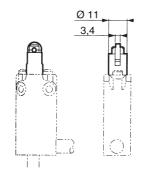
A metal enclosed safety limit switch sealed to IP67 and pre-wired with 1 metre of armoured cable. With 1 N/O + 1 N/C positive break action changeover contacts. Featuring a steel roller plunger actuator.
