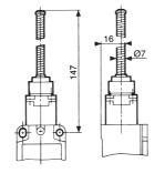
A very reliable, robust safety limit switch with 1 N/O + 1 N/C (positive opening) changeover contacts housed in an all metal construction with a four position metal actuator head. Featuring a flexible metal lever.
