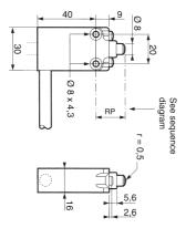
A metal enclosed safety limit switch sealed to IP67 and pre-wired with 1 metre of armoured cable. With 1 N/O + 1 N/C positive break action changeover contacts. Featuring a plain metal plunger actuator.
