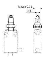
A metal enclosed safety limit switch sealed to IP67 and pre-wired with 1 metre of armoured cable. With 1 N/O + 1 N/C positive break action changeover contacts. Featuring a steel roller plunger actuator.
