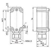
An explosion proof metal bodied limit switch housed in a DIN50041 standard case allowing direct drop to replace non ex standard limit switches. Dual certified for Ex zones 1 and 2 as well as dust zones 21 and 22. Slow action positive break contacts. Available also with 2 N/C positive break contacts and 1 N/O / 1 N/C overlapping positive break.
