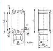
An explosion proof metal bodied limit switch housed in a DIN50041 standard case allowing direct drop to replace non ex standard limit switches. Dual certified for Ex zones 1 and 2 as well as dust zones 21 and 22. Slow action positive break contacts. Available also with 2 N/C positive break contacts and 1 N/O / 1 N/C overlapping positive break.
