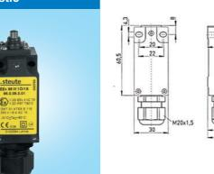
An explosion proof plastic bodied limit switch housed in a DIN50047 standard case allowing direct drop to replace non ex standard limit switches. Dual certified for Ex zones 1 and 2 as well as dust zones 21 and 22. Slow action positive break contacts. Available also with 2 N/C positive break contacts and 1 N/O / 1 N/C overlapping positive break.
