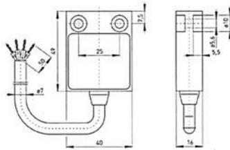
An explosion proof plastic bodied limit switch, certified for Ex zones 1 and 2 as well as dust zones 21 and 22. Slow action positive break contacts.
