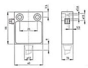
An explosion proof metal bodied limit switch, certified for Ex zones 1 and 2 as well as dust zones 21 and 22. Snap action contacts.
