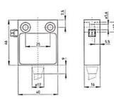
An explosion proof metal bodied limit switch, certified for Ex zones 1 and 2 as well as dust zones 21 and 22. Snap action contacts.
