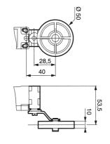
A very reliable, robust limit switch with 1 N/O + 1 N/C positive snap acting changeover contacts housed in a thermoplastic case with a four position metal actuator head. Featuring an offset rotary lever, with left and right action and plastic roller actuator.
