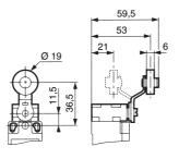
A very reliable, robust limit switch with 1 N/O + 1 N/C positive snap acting changeover contacts housed in a thermoplastic case with a four position metal actuator head. Featuring an offset rotary lever, with left and right action and plastic roller actuator.
