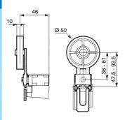
A very reliable, robust limit switch with 1 N/O + 1 N/C positive snap acting changeover contacts housed in a thermoplastic case with a four position metal actuator head. Featuring an adjustable rotary lever, with left and right action and plastic roller actuator.
