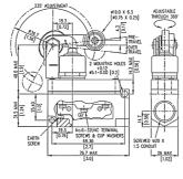
A single pole changeover snap action microswitch with roller level enclosed in a stainless steel housing approved to new ATEX standard. This switch is prefitted with 3 metres of cable.
