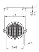
A 63mm diameter reflector specifically designed to be used with reflex sensors. This reflector is fixed on two opposite flanges with two M4 screws.
