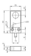
A flush mounted inductive proximity sensor in a quadraform housing, designed to sense ferrous & non-ferrous metals, featuring short circuit & reverse polarity protection. This sensor is ideal for automation & handling applications.
