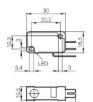
A flush mounted inductive proximity sensor in a V3 style housing. designed to sense ferrous & non-ferrous metals, featuring short circuit & reverse polarity protection. This sensor is ideal for automation & handling applications.
