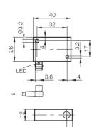
A flush mounted inductive proximity sensor in a quadraform housing, designed to sense ferrous & non-ferrous metals, featuring short circuit & reverse polarity protection. This sensor is ideal for automation & handling applications.
