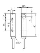
A flush mounted inductive proximity sensor in a 8mm square housing, designed to sense ferrous & non-ferrous metals, featuring short circuit & reverse polarity protection. This sensor is ideal for automation & handling applications.
